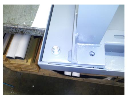
(Picture shown with 1 self-tapping bolt properly in place)
